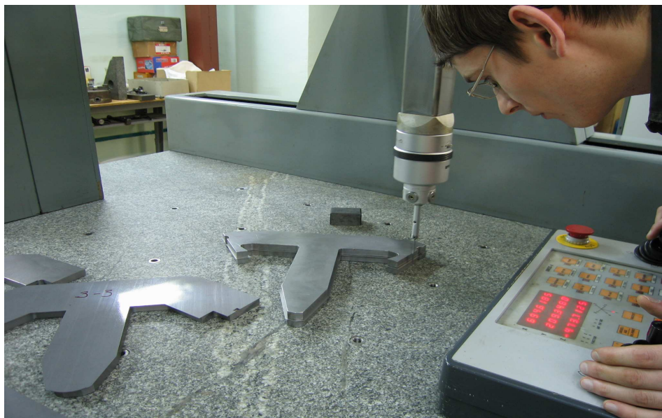
Fig. 8 Measurement in the Budker Institute in Novosibirsk of the thickness of one lamination of the ensemble that constitutes the yoke of a sextupole magnet. The sheet is 0.5 mm thick and here it is sandwiched between two thicker plates for the measurement. The Budker Institute has to provide 260000 similar sheets which have geometrical linear tolerances of \pm 15 \mu\text{m} .
