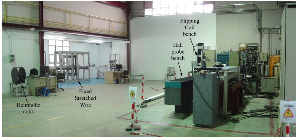
Fig. 6 General view of the magnetic measurements laboratory at CELLS, showing the different measurement benches (from left to right): Helmholtz coils, Fixed stretched wire bench, Hall probe bench and Flipping coil bench. Helmholtz coils and Fixed Stretched wire are used for individual magnet characterization, whereas Hall probe and Flipping coil benches are mainly used for the measurement of larger magnetic structures (electromagnets or Insertion Devices).
